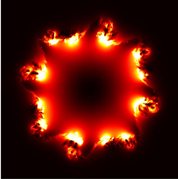
Figure 2: Vortices develop at the interface between counter-rotating flows, simulated on a multi-resolution grid using 17 levels of detail. Retaining the sparse structure during rendering maintains an effective compression ratio of  $500x$  and allows each timestep to be converted and rendered in less than one second.
