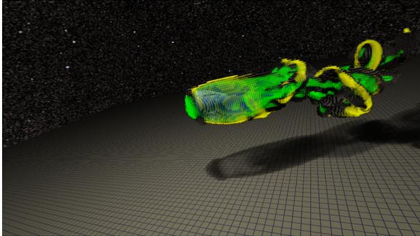
Figure 3: Ray-traced image from NVIDIA OptiX™, using refraction to visualize wake formation around a capsule during late re-entry (Mach = 0.33)
