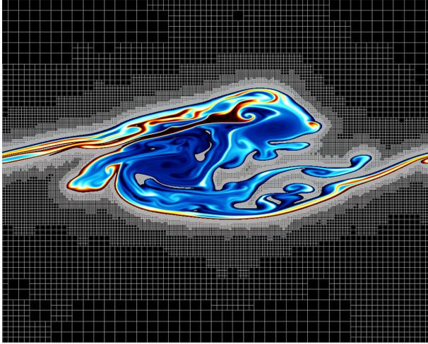
Figure 1: Periodic shear flow simulation ( $Re = 80,000$ , 14 levels of resolution), colored by fluid density and showing wavelet mesh refinement.
