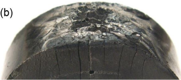
(b) Pore pressure-induced crack in PR-CB (Natali et al. 2016)
