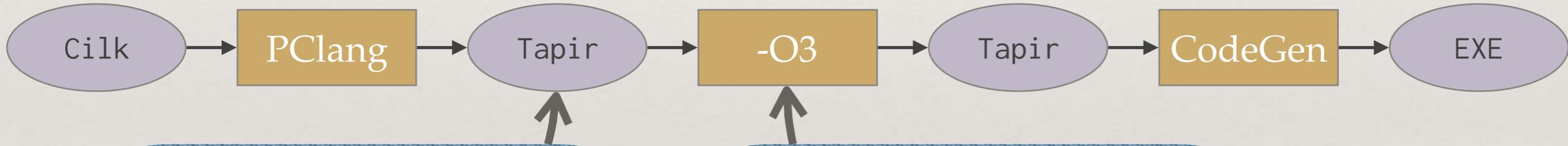
Tapir adds **three instructions** to LLVM IR that encode **fork-join parallelism**.
